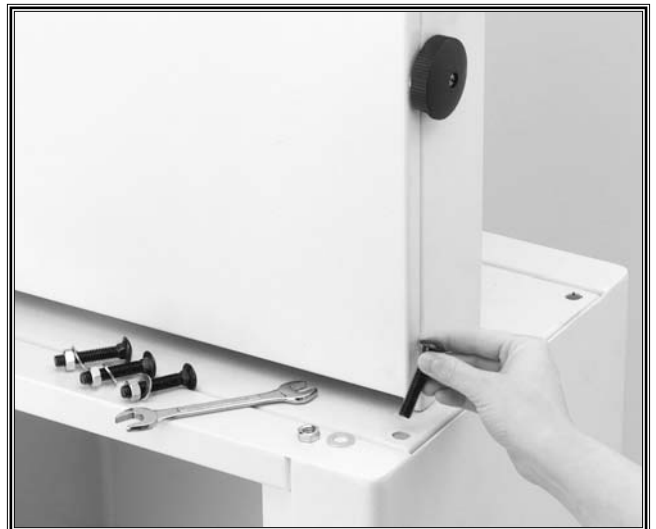
Figure 13. Securing bandsaw body.
